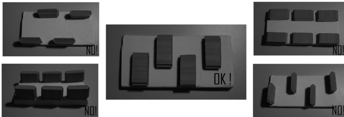
Figure 4: Correct or wrong placing of the bricks in the quarter-deck (Cristini-Ruiz Checa)
